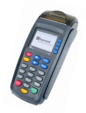
The PAX S90 is a 3G wireless terminal compatible with Rogers, Telus and Bell networks. It does not support WIFI connectivity. Contact your Payment Service Provider for SIM card and data plan.
